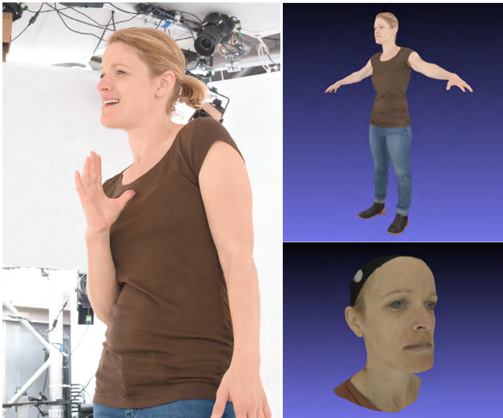
Figure 4. The generation of the 3D avatar model. Left: The participant inside a photogrammetry cage. Right top: The 3D avatar model generated from photogrammetry capture. Right bottom: Light Stage facial scans used for reference for avatar construction.
